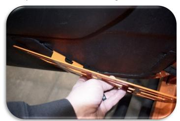
Align the two holes in the GhostFire Industries Molle door panel with the two holes that are used for mounting the door strap bracket.
