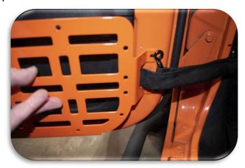
Reinstall the two screws through the door strap bracket and GhostFire Molle door panel. Hand tighten both screws.
